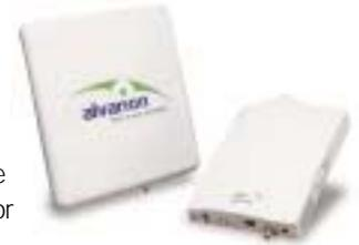
The outdoor unit comprises a radio module with either an integrated flat panel antenna or a connector for an external antenna.
